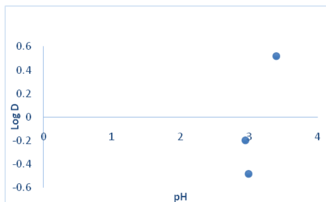
Fig. 3: Extraction plot of 200 mg/l U(VI) ion with solutions of 0.05 M HTCP in chloroform from buffer solutions containing 0.1 M SO_4^{2-} at 25 °C
