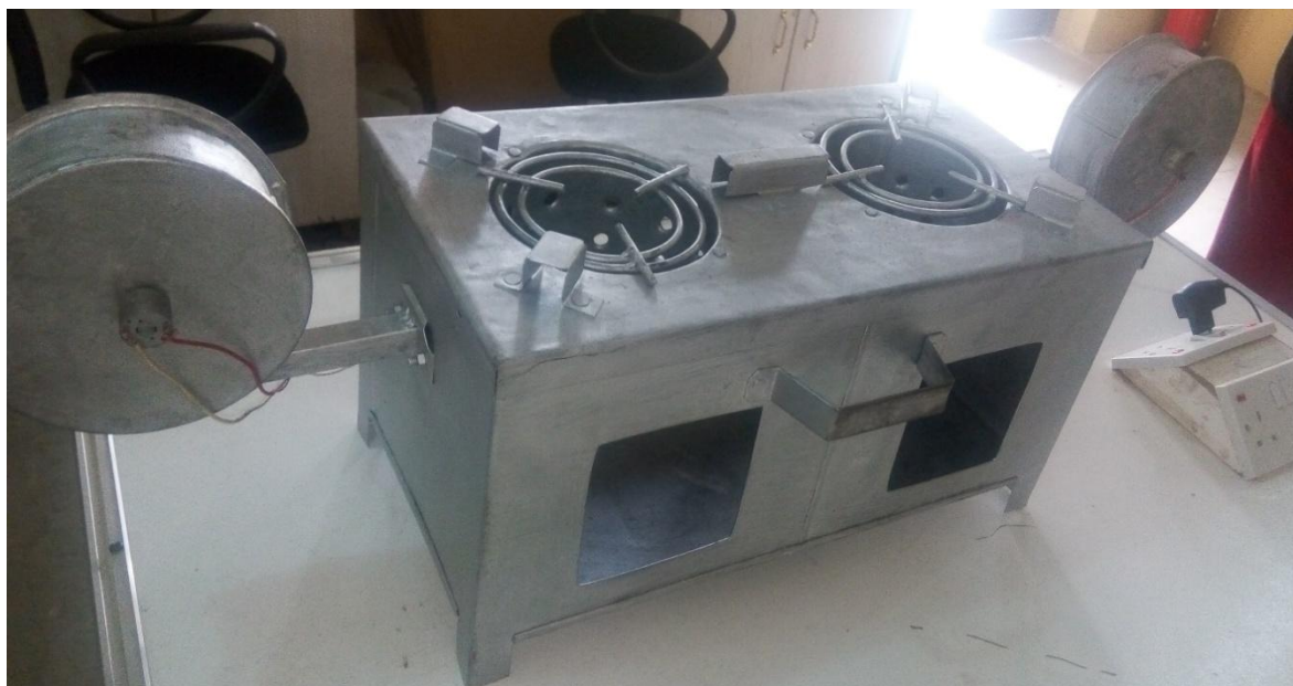
Fig.2.The constructed two-pot forced air charcoal stove
