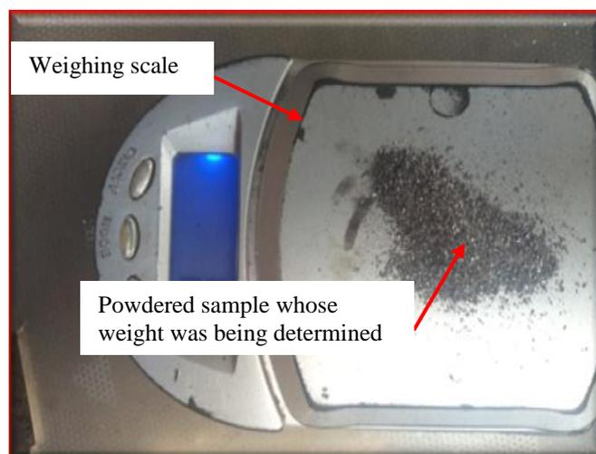
Plate I: Process of weight-determining the required amount of metal powder
