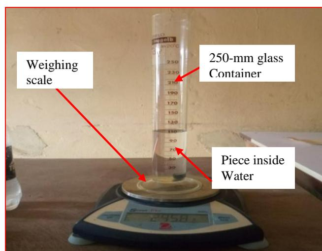
Plate V: Process of determining mass and volume of an alloy rod piece in the laboratory
