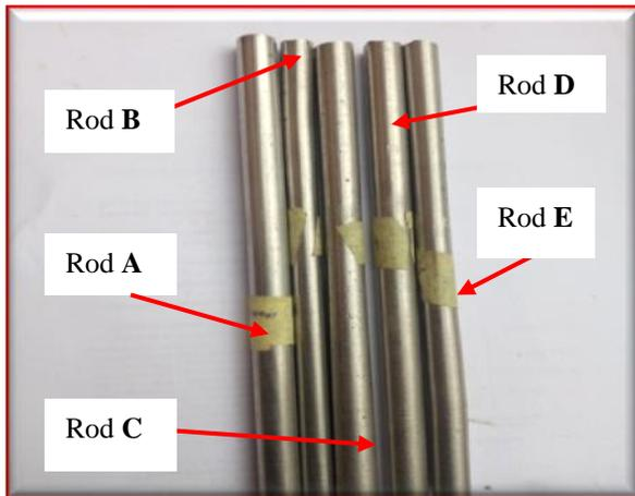
Plate II: The cast-fabricated Al-Si-Fe alloy rods after trimming their surfaces
