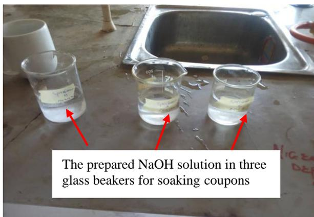
Plate IV: Coupons from groups A, B, and C under immersion in NaOH solution in glass beakers
