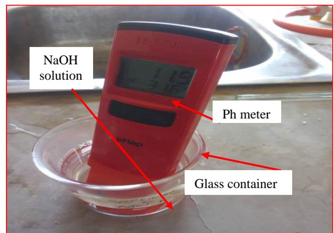
Plate III: Process of determining the Ph of the prepared NaOH solution in the laboratory using a Ph meter
