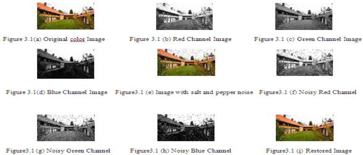
Figure 3.1 House Image with salt and pepper noise and finally restores the original image with Median Filter
