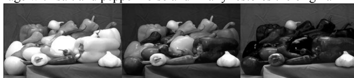
Figure 1.2 Pepper (a) Image of Kuwahara Filter (b) Image of Hybrid Filter (c) Image of Weiner Filter
