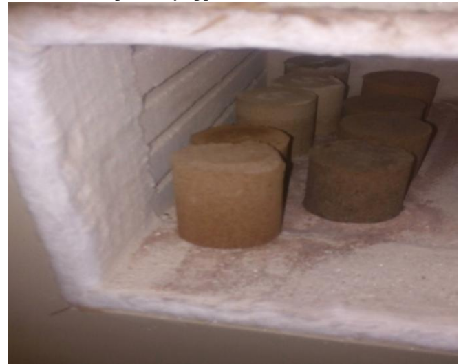
Figure 1: Photograph of produced samples in Furnace for baking
