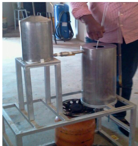
Plate 1: The Stainless Steel Biodiesel Reactor
